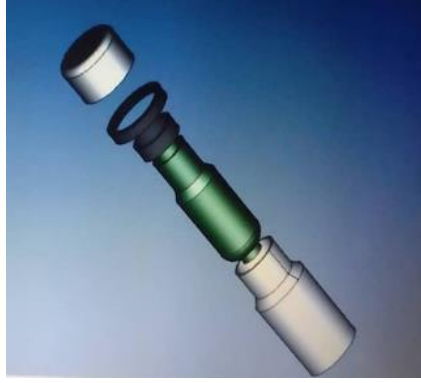
Figure 1: Exploded View of Thermos Flask Design
